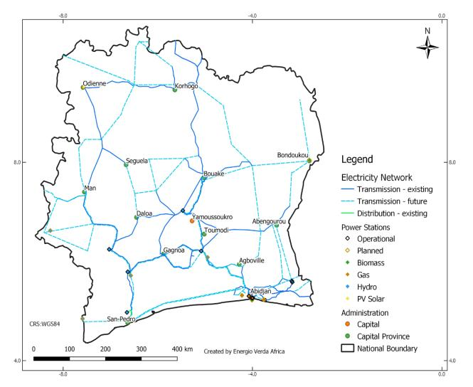
Figure 3: Electricity Transmission and Distribution Network<sup>61</sup>
