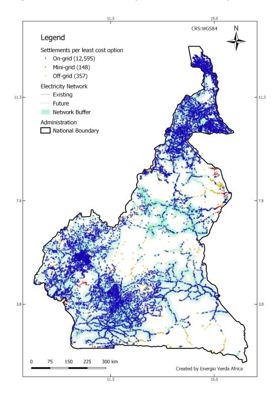
Figure 5: Distribution of Settlements by Least-Cost Electrification Option, 2030<sup>61</sup>
