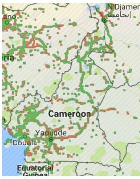
Green: Strong Signal (>-85dBm) Red: Weak Signal (<-99dBm) Source: Open Data Signal
