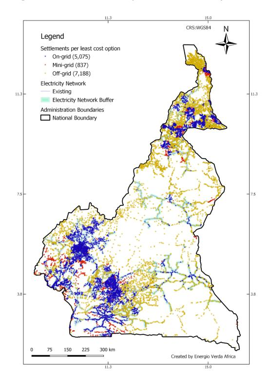
Figure 4: Distribution of Settlements by Least-Cost Electrification Option, 2023<sup>60</sup>
