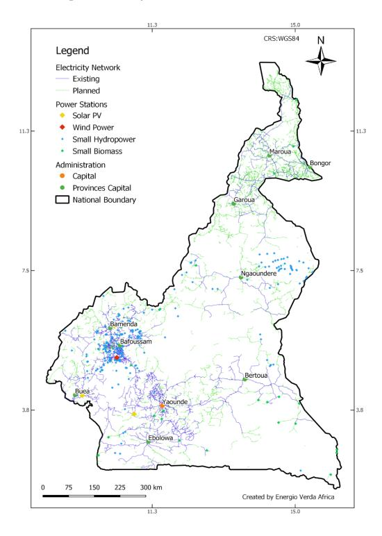
Figure 1: Electricity Transmission and Distribution Network<sup>51</sup>
