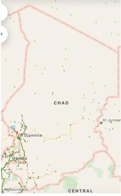
Green: Strong Signal (>-85dBm) Red: Weak Signal (<-99dBm) Source: Open Data Signal
