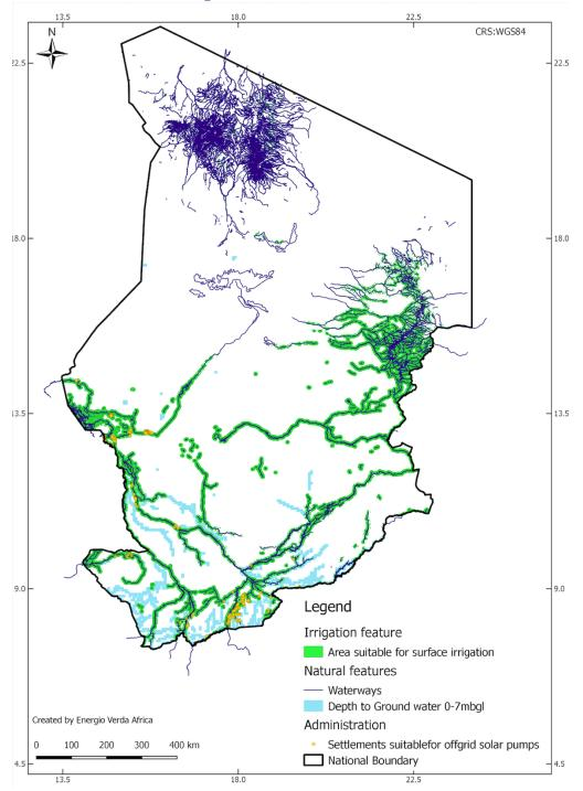
Figure 29: Area Suitable for Surface Irrigation and Identified Settlements Suitable for Off-Grid Solar Pumps
