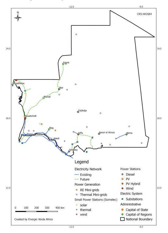
Figure 2: Electricity Transmission and Distribution Network<sup>61</sup>
