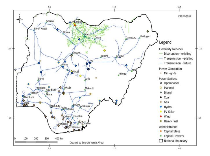
Figure 5: Electricity Transmission and Distribution Network<sup>62</sup>
