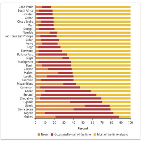
Figure 10: Reliability of Grid Electricity in Connected Households in Africa<sup>139</sup>
