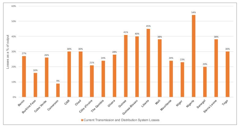
Figure 8: Transmission and Distribution System Losses in West Africa and the Sahel, 2016<sup>137</sup>
