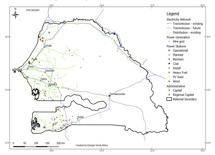
Figure 3: Electricity Transmission and Distribution Network<sup>57</sup>
